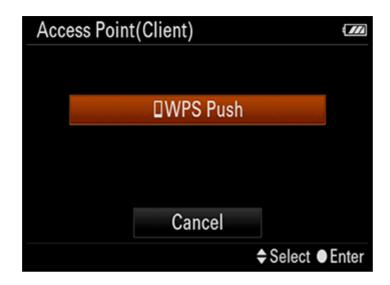
If the screen above does not appear, display it by selecting MENU > (Network) > [Ctrl w/ Smartphone] > [Access Point (Client)] > [OK].
